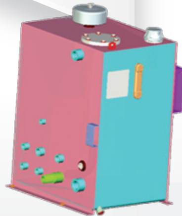
Current State 40 Gallon Hydraulic Tank
